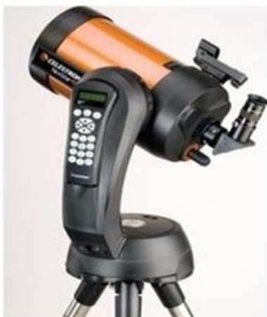
LEFT: A Schmidt-Cassegrain telescope with an altazimuth mount, motors, and go-to computer
